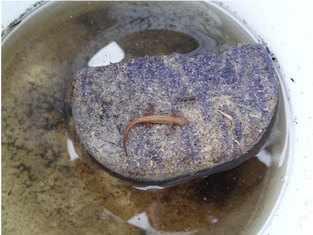
Figure 6. Sponges were used within bucket traps as safeguards to prevent drowning as well as to retain moisture if buckets went dry. One of three captured emigrating striped newt efts sits atop a sponge in a pit fall trap.
