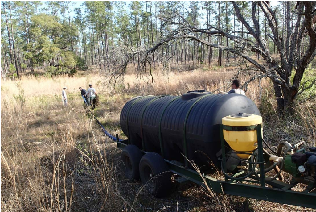
Figure 4. A 1000-gallon water tank on a trailer. Pulled by a large 4x4 fire truck, this tank and trailer combination was our water transport medium from source pond to recipient pond.
