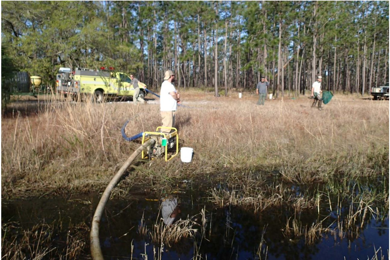
Figure 3. Water extraction from source Pond 178. A gas-powered suction pump removed water from the source pond and delivered it into a nearby 1000-gallon water tank.
