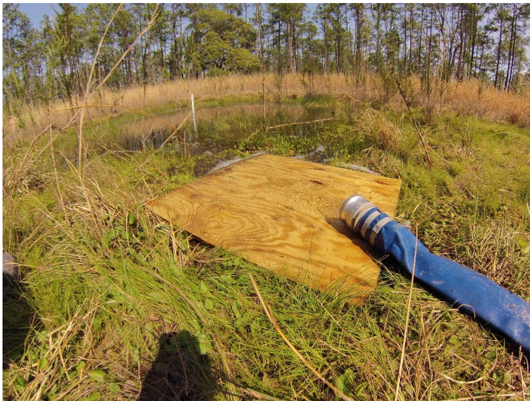
Figure 5. Water delivery into recipient Pond 18. A gas-powered pump sucked water out of a nearby 1000-gallon tank and delivered it through a hose into our recipient pond. Water discharged through the hose onto a 1.5m x 1.5m flat plywood. The plywood acted to shield the pond edge from the formation of a hydraulically blasted out hole.
